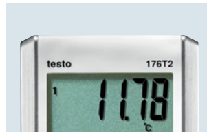
Large, clear display for showing measurement values (testo 176 T2 only)
