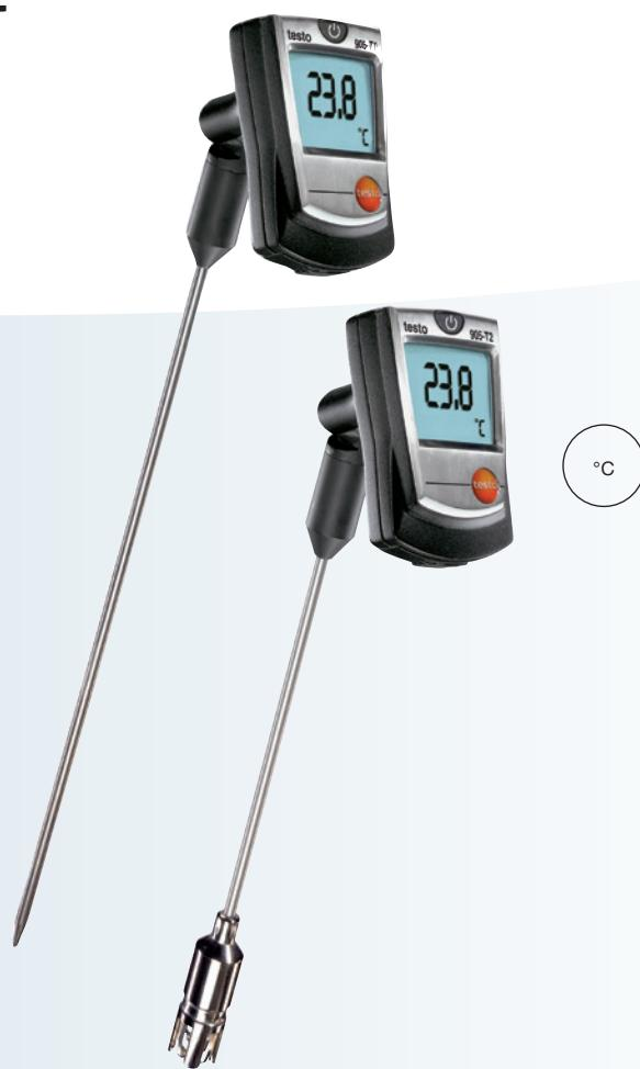
The testo 905-T1 is a particularly fast penetration thermometer with a broad measuring range of -50 to +350 °C, in the short term even up to +500 °C (1 to 2 minutes). The measuring instrument has a professional industrial sensor (thermocouple Type K). It has an excellent level of accuracy, especially in the upper measuring range. The testo 905-T2 is a surface thermometer with a broad measuring range of -50 to +350 °C, in the short term
